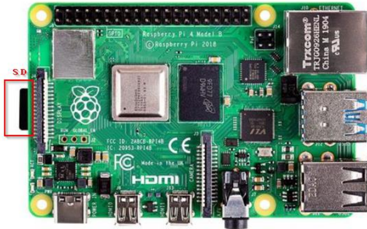
Figure 2-5: Raspberry Pi uses an SD card to boot Embedded Linux
