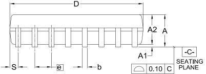
Dimensions (inch dimensions are derived from the original mm dimensions)
