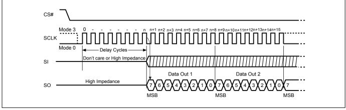
Note: If FBSD = 11, delay cycles is 13 and n is 12. If FBSD = 10, delay cycles is 11 and n is 10. If FBSD = 01, delay cycles is 9 and n is 8. If FBSD = 00, delay cycles is 7 and n is 6.
