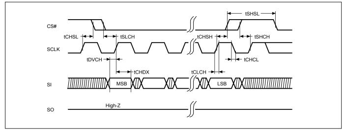
Figure 3. Serial Input Timing (DTR mode)
