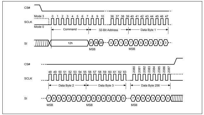
Figure 59. 4 x I/O Page Program (4PP4B) Sequence (SPI Mode only)
