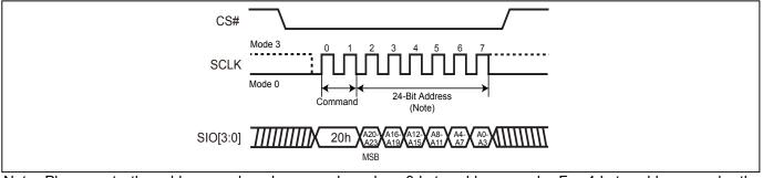
Note: Please note the address cycles above are based on 3-byte address mode. For 4-byte address mode, the address cycles will be increased.
