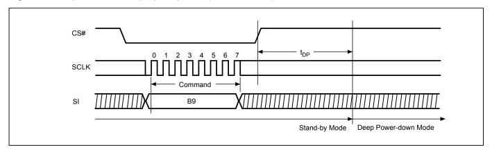
Figure 23. Release from Deep Power-down (RDP) Sequence (Command AB)
