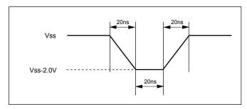
Figure 4. Maximum Positive Overshoot Waveform
