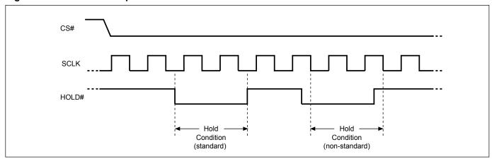
The Serial Data Output (SO) is high impedance, both Serial Data Input (SI) and Serial Clock (SCLK) are don't care during the HOLD operation. If Chip Select (CS#) drives high during HOLD operation, it will reset the internal logic of the device. To re-start communication with chip, the HOLD# must be at high and CS# must be at low.
