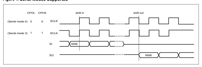
Figure 1. Serial Modes Supported
