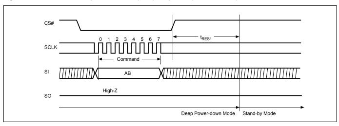
Figure 24. Read Electronic Signature (RES) Sequence (Command AB)
