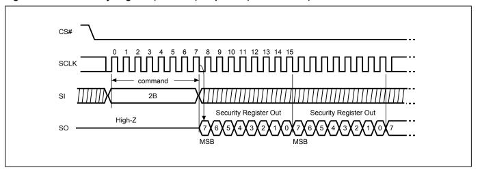
Figure 28. Write Security Register (WRSCUR) Sequence (Command 2F)
