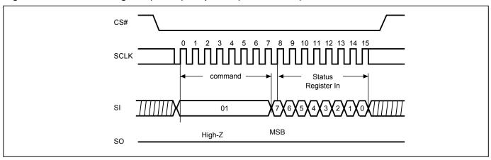
Figure 15. Read Data Bytes (READ) Sequence (Command 03)
