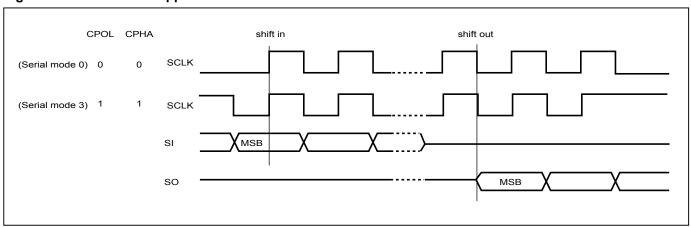
Figure 1. Serial Modes Supported
