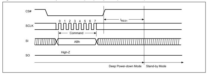
Figure 40. Read Electronic Manufacturer & Device ID (REMS) Sequence (Command 90/EF/DF)
