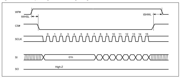
Figure 19. Write Enable (WREN) Sequence (Command 06)
