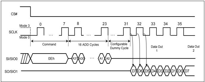
**Note:** Configuration Dummy cycle numbers will be different depending on the bit6 & bit7 (DC0 & DC1) setting in configuration register.
