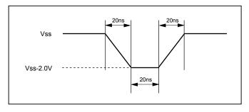
Figure 120. Maximum Positive Overshoot Waveform
