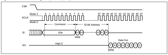
Figure 107. Write DPB Register (WRDPB) Sequence
