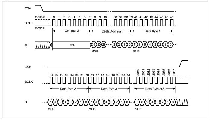
Figure 68. 4 x I/O Page Program (4PP4B) Sequence (SPI Mode only)
