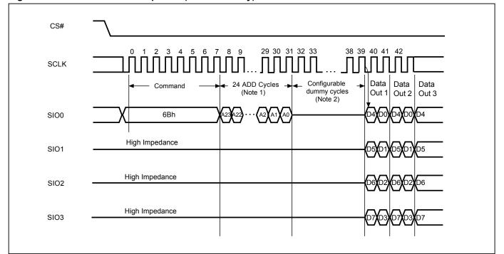
Figure 39. Quad Read Mode Sequence (SPI Mode only)
