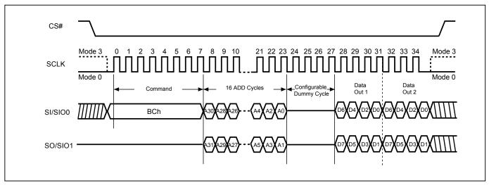
**Note:** Configuration Dummy cycle numbers will be different depending on the bit6 & bit7 (DC0 & DC1) setting in configuration register.
