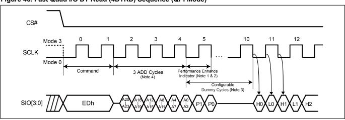
Figure 45. Fast Quad I/O DT Read (4DTRD) Sequence (QPI Mode)
