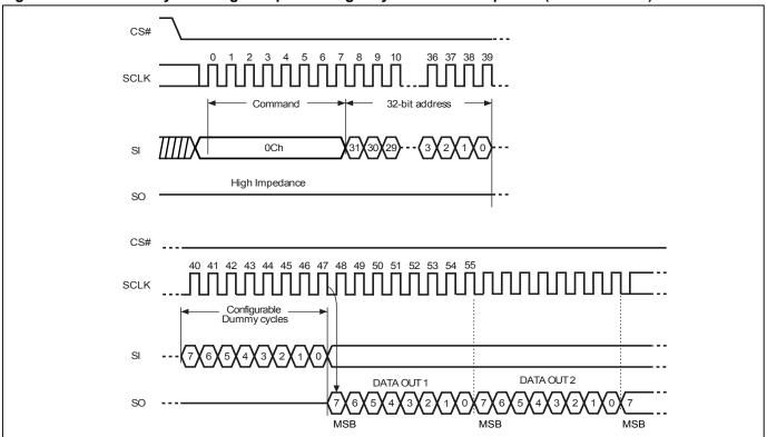
**Note:** Configuration Dummy cycle numbers will be different depending on the bit6 & bit7 (DC0 & DC1) setting in configuration register.
