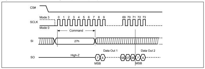
Figure 109. Write Password Register (WRPASS) Sequence
