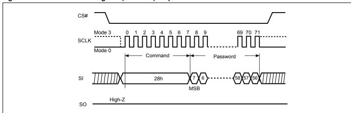
Figure 110. Password Unlock (PASSULK) Sequence
