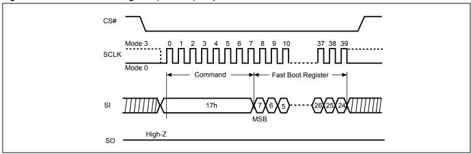
Figure 79. Erase Fast Boot Register (ESFBR) Sequence
