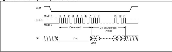
Note: Please note the address cycles above are based on 3-byte address mode. For 4-byte address mode, the address cycles will be increased.
