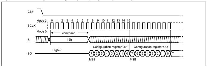
Figure 28. Read Configuration Register (RDCR) Sequence (QPI Mode)
