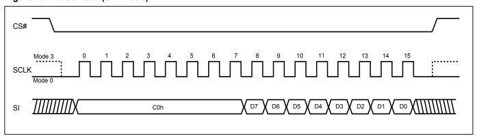
Figure 74. Burst Read (QPI Mode)
