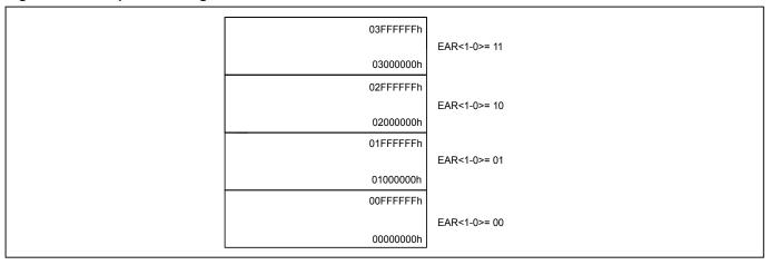
When under EAR mode, Read, Program, Erase operates in the selected segment by using 3-byte address mode.
