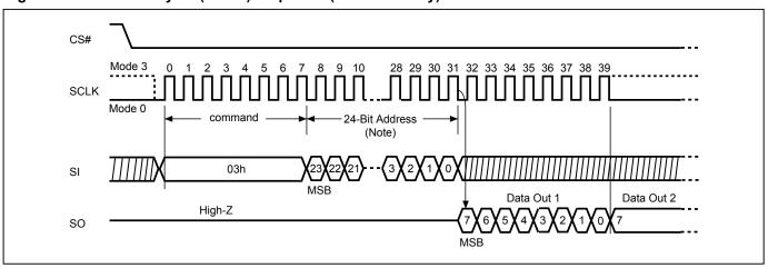
Figure 35. Read Data Bytes (READ) Sequence (SPI Mode only)
