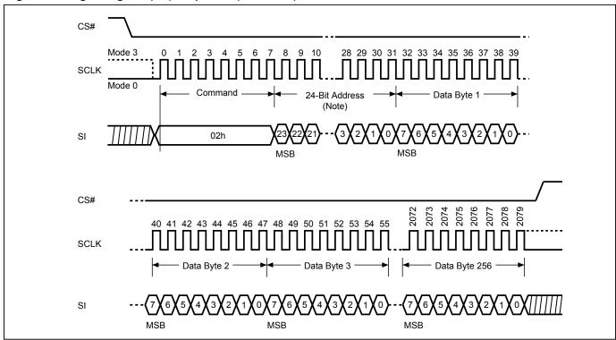
Note: Please note the address cycles above are based on 3-byte address mode. For 4-byte address mode, the address cycles will be increased.
