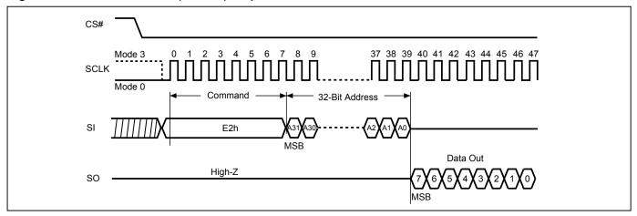
Figure 104. SPB Erase (ESSPB) Sequence
