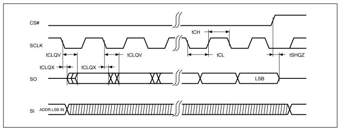
Figure 5. Output Timing (DTR mode)
