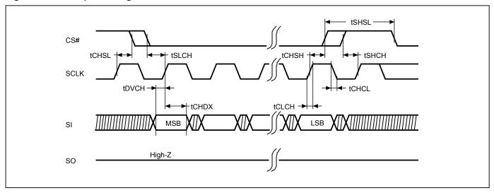
Figure 3. Serial Input Timing (DTR mode)
