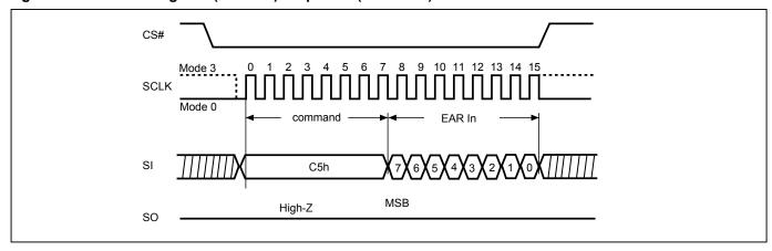
Figure 7. Write EAR Register (WREAR) Sequence (QPI Mode)
