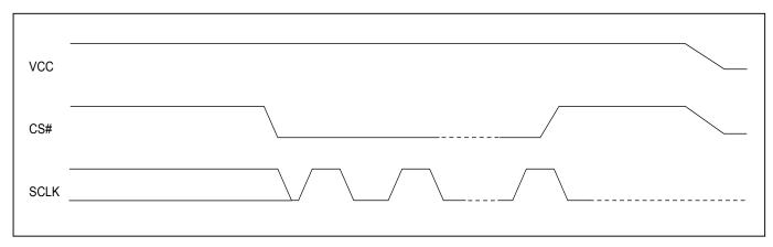
Figure 34. Power-up Timing
