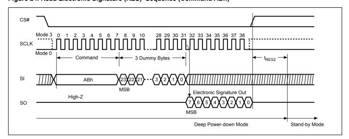
Figure 24. Read Electronic Signature (RES) Sequence (Command ABh)
