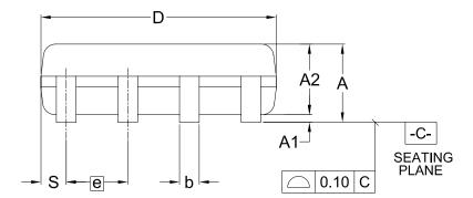
Dimensions (inch dimensions are derived from the original mm dimensions)
