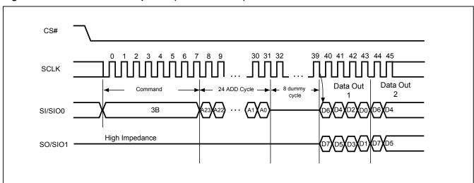
Figure 16. Dual Read Mode Sequence (Command 3Bh)
