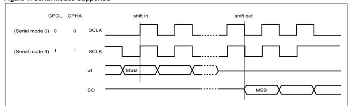
Figure 1. Serial Modes Supported
