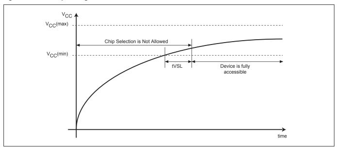
Note: VCC (max.) is 3.6V and VCC (min.) is 3.0V.
