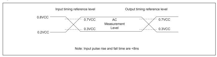
Notes: Rise time means 0.2VCC to 0.8VCC; Fall time means 0.8VCC to 0.2VCC.
