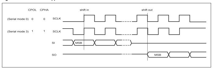
Figure 1. Serial Modes Supported
