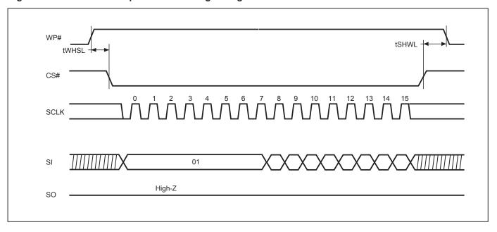
Figure 9. Write Enable (WREN) Sequence (Command 06)
