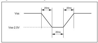
Figure 3. Maximum Positive Overshoot Waveform
